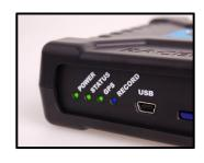
7. The REC LED will illuminate when recording, when the vehicle comes to a stop, it will flash as the file is closed.
