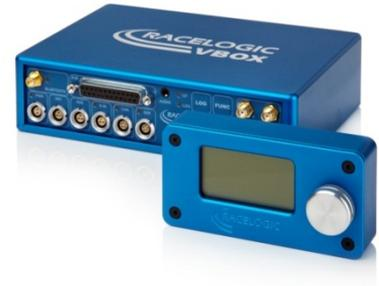
The new VBOX3i Dual Antenna (VBOX3i SL) uses two antennas placed a fixed distance apart to capture vehicle dynamics (along the vehicle for pitch and across the vehicle for roll). By utilising both the GPS and Russian GLONASS constellations, RMS accuracies of up to 0.04° for slip and 0.028° for pitch can be achieved.
