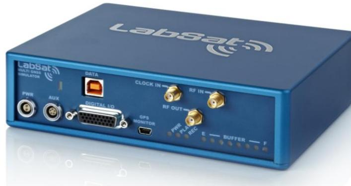
Responding to the increasing need for developers of GNSS devices to be able to test GLONASS enabled systems, Racelogic have launched LabSat 2: a dual channel unit capable of recording, replaying, and simulating GLONASS data in addition to GPS.
