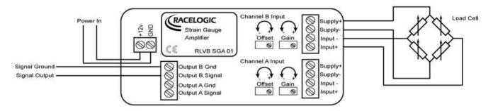
The Strain Gauge Amplifier can also be used in half-bridge and quarter-bridge applications. Please refer to the user manual for more information.
